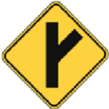
Side road enters highway ahead at an angle.
