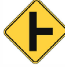
Side road enters highway ahead.
