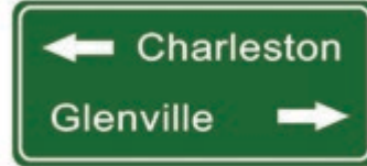
Found in front of intersections, these signs show the direction to cities.
