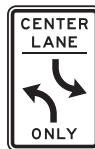
Two-way Left Vehicles traveling in either direction can use the center lane to turn left.
